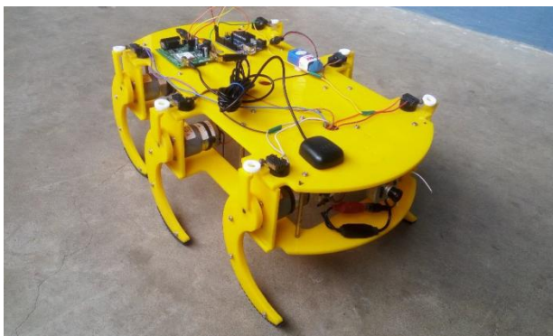
Fig. 5. Robot fitted with GPS & GSM module
