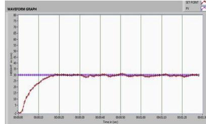
**Fig.6 Simulation Result Of FLC Controller Implemented Forconical Tank Using Lab VIEW**
