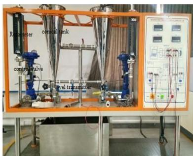
**Fig.1 Experimental setup of conical tank system**
