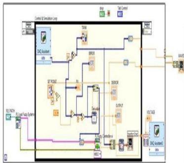
**Fig.4 Block Diagram Of FLC Implemented Using Labview**
