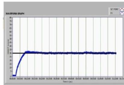
**Fig.7 Simulation Result Of Adaptive Fuzzy PID Controller Implemented For Conical Tank Using Labview**
