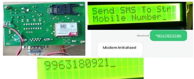
Fig4.GSM based processing operations and display information about mobile number
