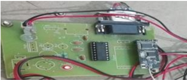
Fig6. ZIGBEE Module Interfaced in the Hardware
