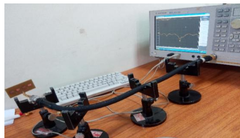
Figure 16. Measurement of S11 with Network Analyzer
