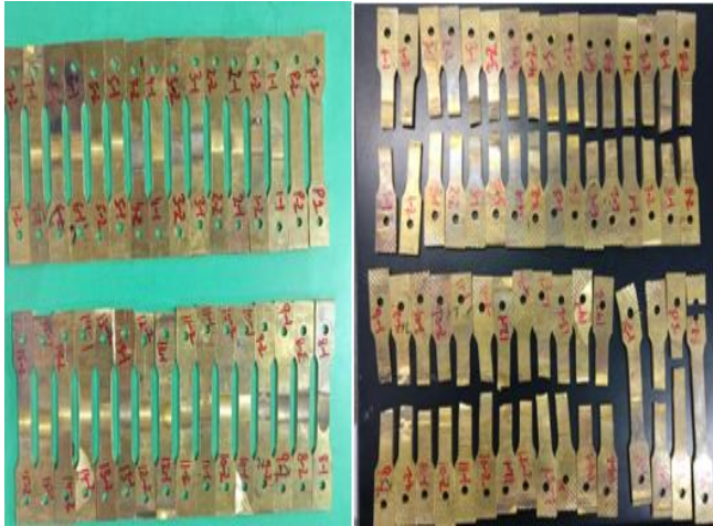
Figure 5: Tensile Test Specimens before and After Test
