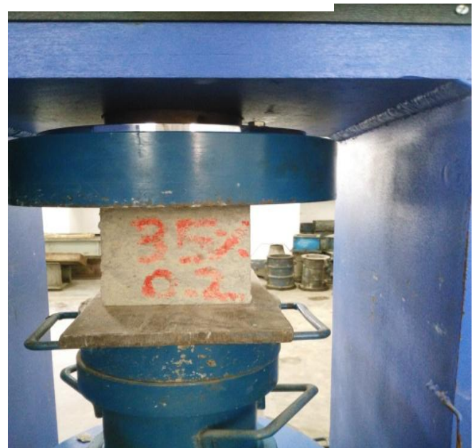
Fig.1. Cube Compression testing
