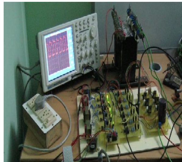
Fig.12.Experimental setup of SPWM controller
