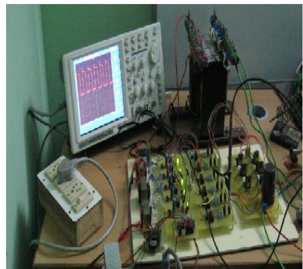
Fig.12.Experimental setup of SPWM controller
