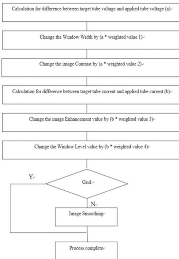
Figure 4. Flowchart for applying the image adjustment filter
