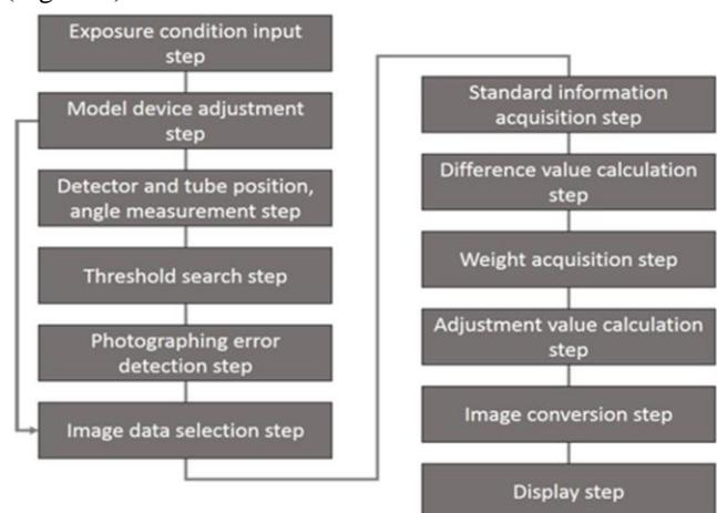
Figure 1. Flowchart of processing method of output image performed by radiography simulation system
