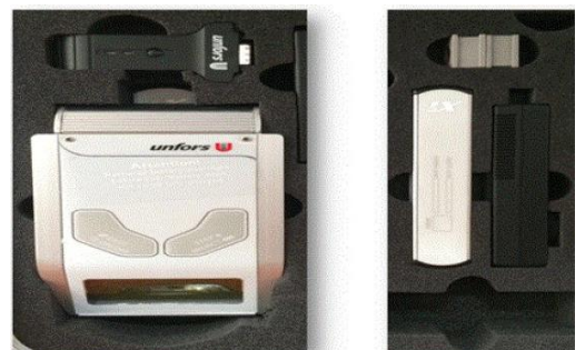
Figure 2.Unfors's Xi R/F & MAM Detector as dosimeter, which was calibrated in June 2017
