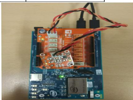
Figure 5. IoT device with Edison board and temperature sensor
