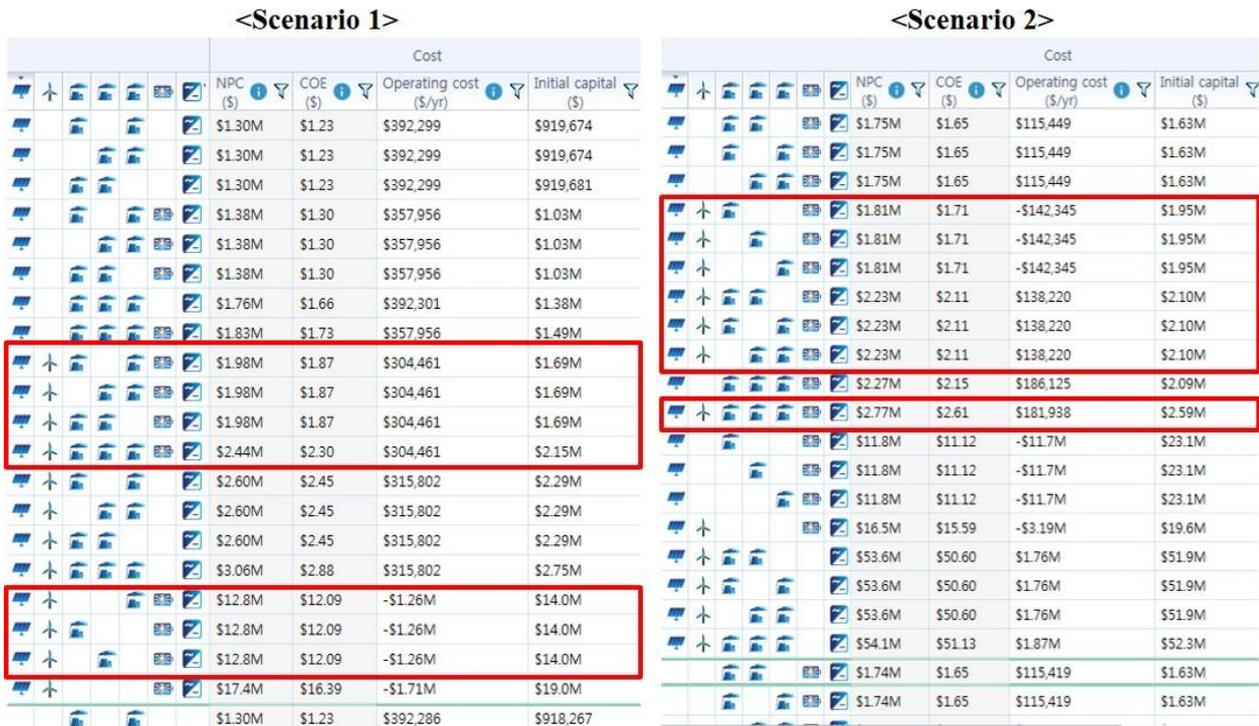
Fig 9. Simulation results of HOMER PRO (optimal operation combination)
