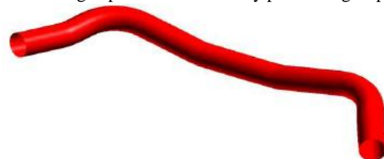
Figure 6. The six-bending tube shape used for hydroforming
