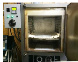
Post curing of the laminate
