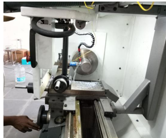
Figure 2: Turning of AISI 3415 steel in a flooded condition
