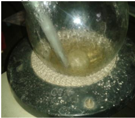
Fig 2.3 Adding monohydrate to graphene oxide and then heated
