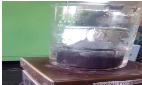
Fig 2.1 Magnetic stirring of Graphite with H 2 SO 4 at ice bath (0-5°C)
