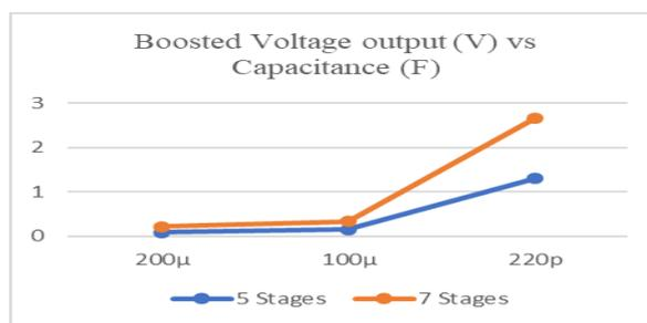
**Figure 6: Boosted output voltage against capacitance value at 1.8 GHz**
