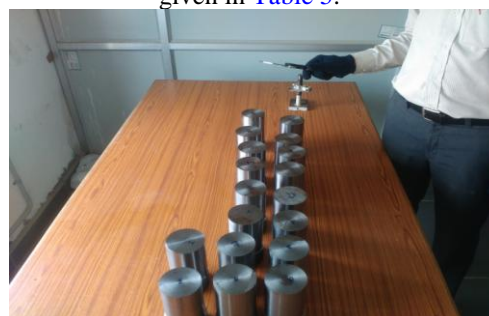
Figure 4: Machined steel alloy AISI 52100 components
