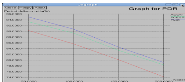
Figure.5 Packet Delivery Ratio Vs Number of Nodes
