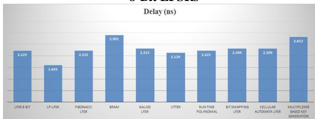
Figure-41: Delay (ns) comparison for Different 8-Bit LFSRs
