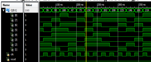
Figure 36 Cellular Automata LFSR using XOR Logic
