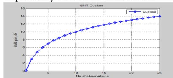
**Figure 4: As the number of observations get increased the SNR gain increases effectively**
