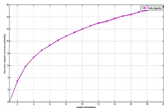
Figure 8: SNR is increased with number of observations
