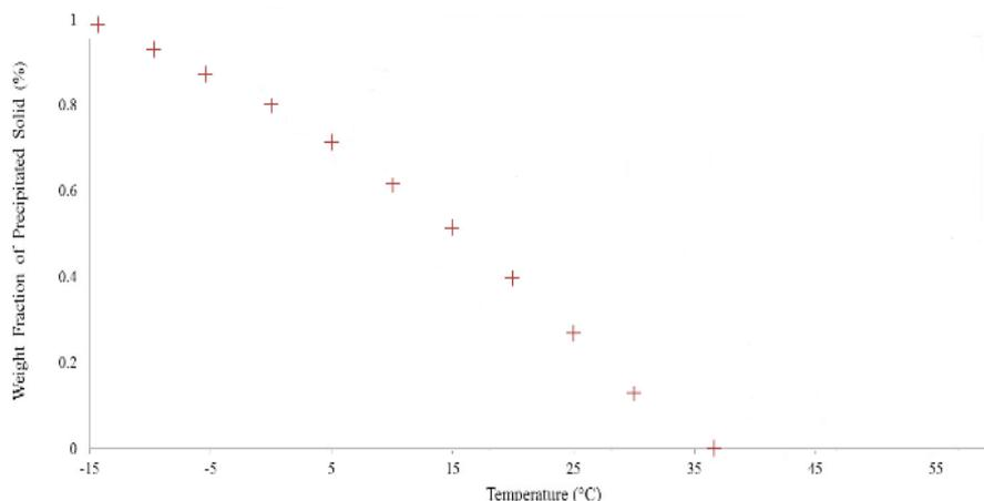
Fig. 3 Precipitated Solid (%) vs. Temperature Graph
