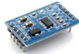
Fig. 1 Accelerometer sensor of stair climbing robot
