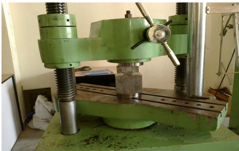
Fig. 4.1 MAF die assembly fitted in the UTM machine
