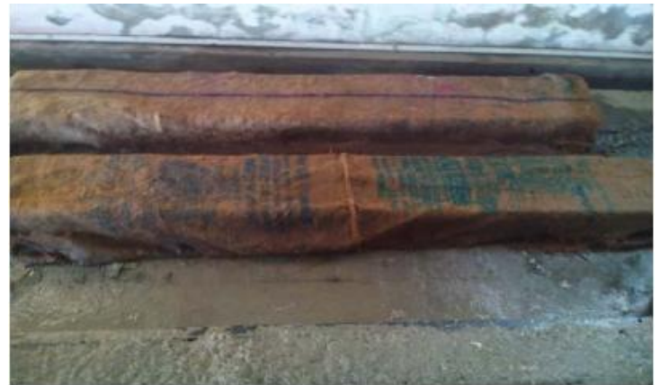
Fig 3. Curing of Specimens
