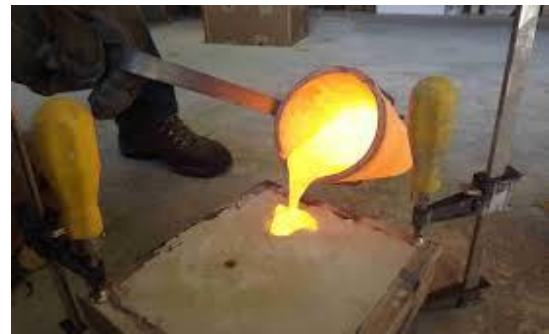
Figure 12: Pouring of molten metal to the cavity
