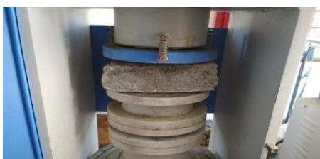
Fig 8: Brick placed under compression testing machine
