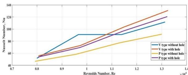
**Fig 4. Nusselt number Vs Reynold's number for aluminium for different configurations**
