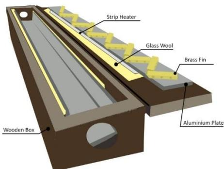
Fig 1. b Experimental Setup (Brass)
