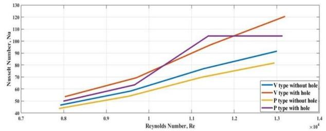
**Fig 5. Nusselt number Vs Reynold's number for Brass for different configurations**
