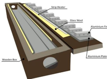
Fig 1. a Experimental Setup(Al)
