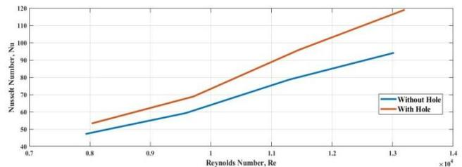
**Fig 7. Nusselt number Vs Reynold's number comparing fins with hole and fins without holes**
