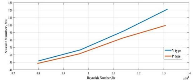
**Fig 6. Nusselt number Vs Reynold's number comparing P-type and V-type configurations**
