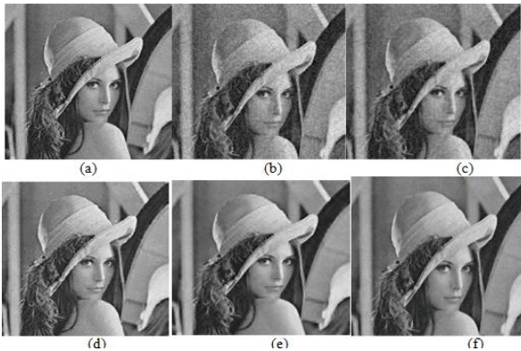
Figure.4 Results of Lena image, (a) Noisy image, denoised through (b) WT-SVD-DF, [24], (c) WT-IC [25], (d) DT-CWT-PG [38], (e) DT-CWT-GPG [45], and (f) Proposed
