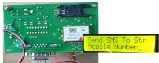
Fig4. GSM/GPRS Used For Sending And Receiving The Information
