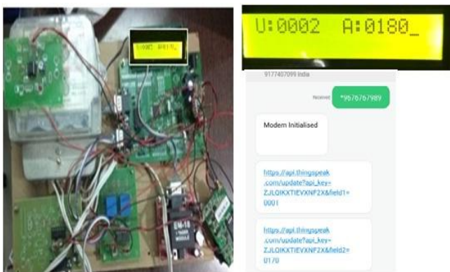
Fig6: Experimental hardware arrangement and information display about number of units consumption along with initialization process
