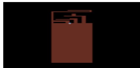
Fig1 PIFA antenna design using ADS
