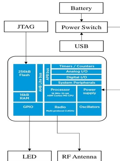
Fig. 3 The Hardware Design Block Diagram of The Transmitter
