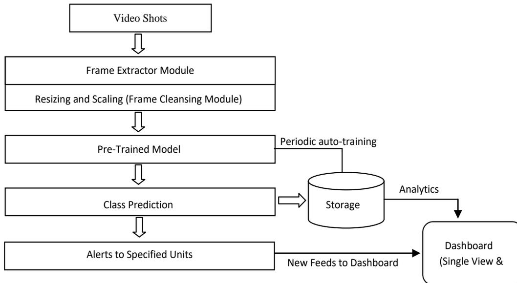
Fig 1.2 S-TVDS Workflow Diagram
