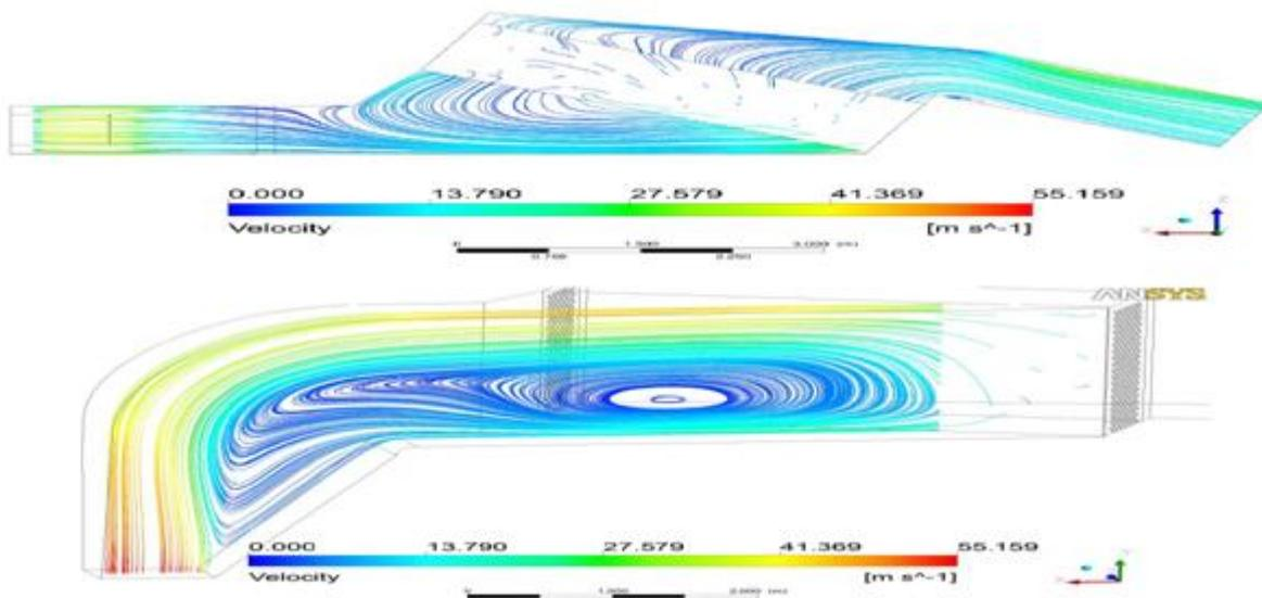
Fig.5 Velocity streamline contours of Air Preheater duct
