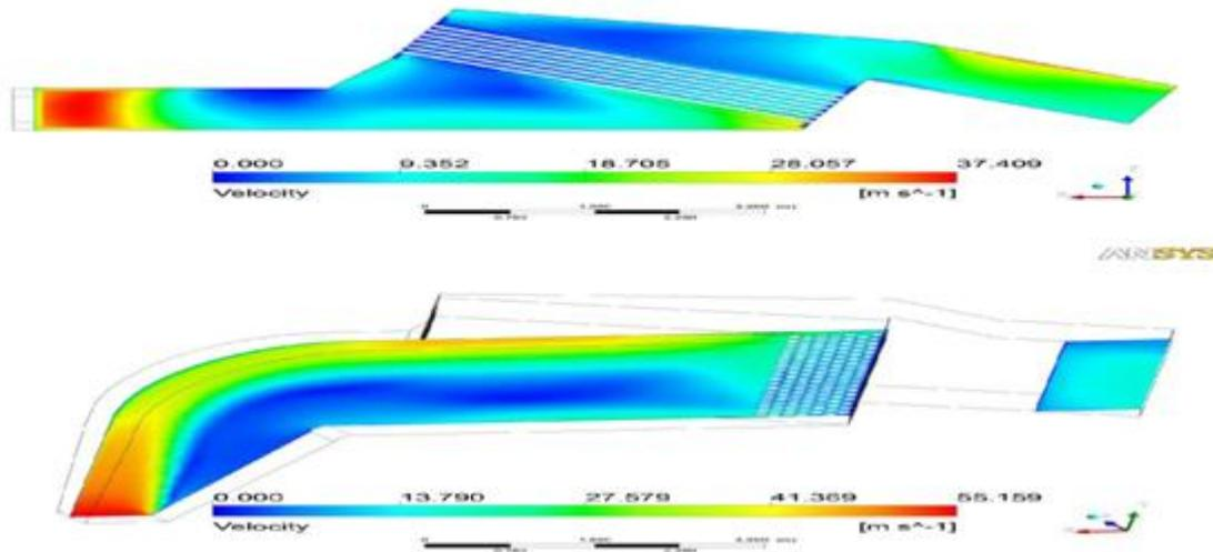
Figure 4. Velocity contours of Air Preheater duct
