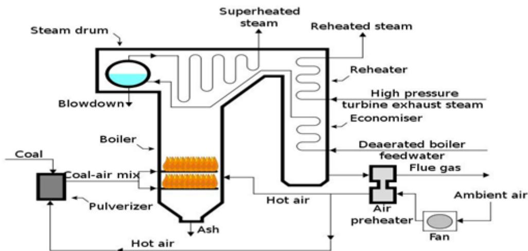
Fig.1. Diagram of coal fired steam generator with air preheater
