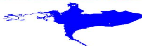
Fig.3(a) False color composite and (b) Extracted water spread on May 13, 2015 (Res. Level: 505.08 m)
