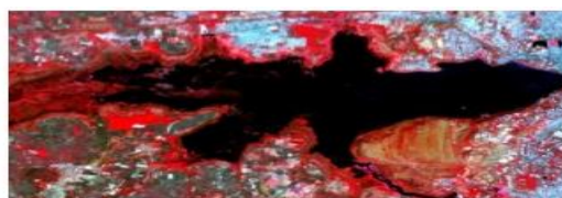
Fig 5 (a) False color composite and (b) Extracted water spread on Jun 11, 2014 (Res. Level: 506.07 m)
