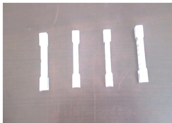
Fig.5 Samples prepared through End Milling Process for various testing.
