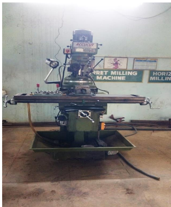
Fig. 3 Vertical Milling Machine Used for FSW
