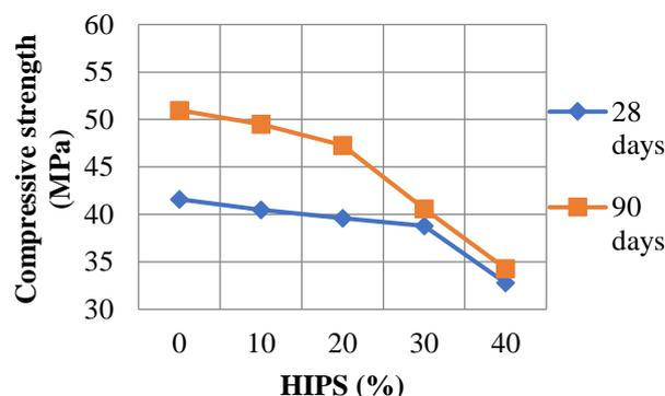
Figure 6: Compressive strength variations with different % of HIPS aggregate
