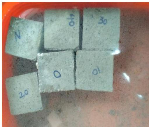
Figure 2: SCC specimens with HIPS in water tank
