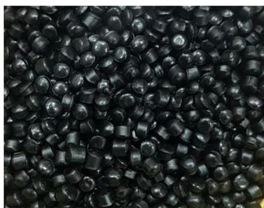
Figure 1: High impact polystyrene granules
