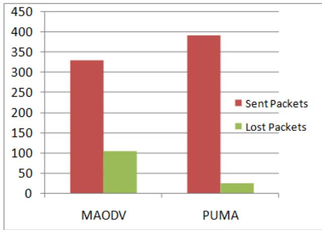
Figure 1.8 Packet Loss (Infra. Less)
