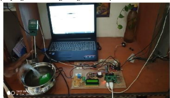
Fig 7. IoT Model developed for calculating the Water Quality
