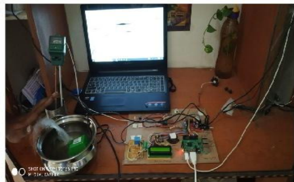
Fig 7. IoT Model developed for calculating the Water Quality
