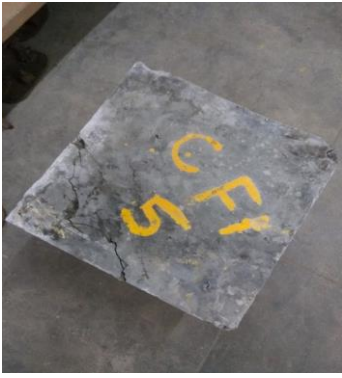
Figure 9 crack observed on two sides supported slab specimen without steel fibre
