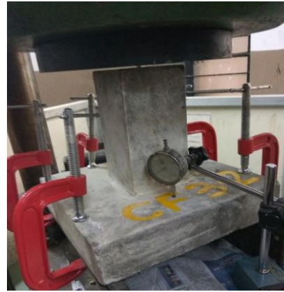
Figure 2 Test setup for slab specimen
