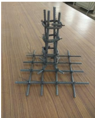
Figure 1 Reinforcement of the test specimen
