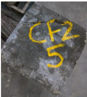
Figure 12 crack observed on two sides supported slab specimen with 0.3% of steel fibre
