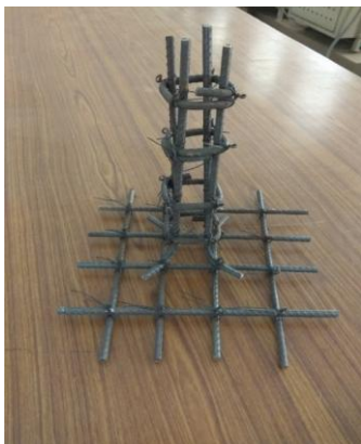
Figure 1 Reinforcement of the test specimen
