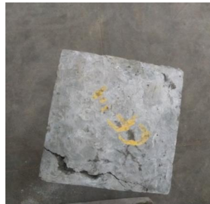
Figure 7 crack observed on four sides supported slab specimen without steel fibre
