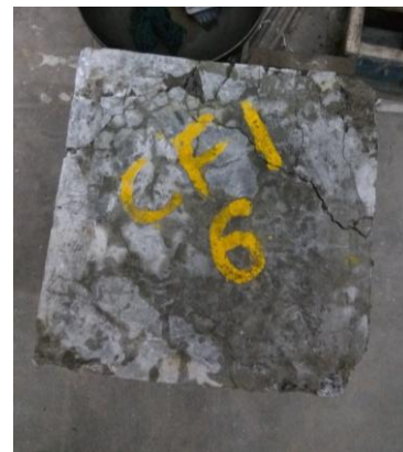
Figure 8 crack observed on three sides supported slab specimen without steel fibre
