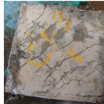
Figure 15 crack observed on two sides supported slab specimen with 0.4% of steel fibre
