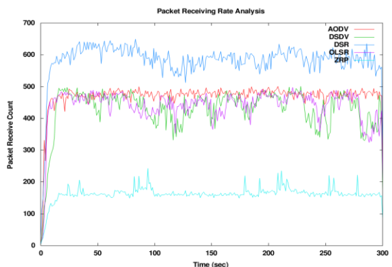
Figure 10: Packet receiving / delivery rate analysis for 20 nodes.
