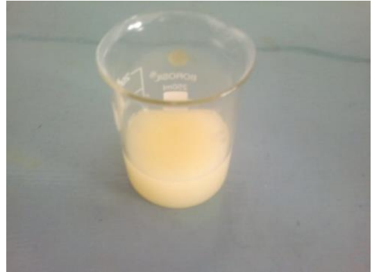
Fig. 2 \text{SnCl}_2 and \text{HCl} solutions after 72 hours of aging
