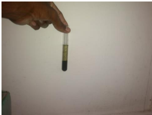
Fig. 5 CNTs in a test tube after centrifugation
