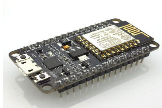
Fig.2: NodeMcu has a interface between hardware and Mobile Application.
