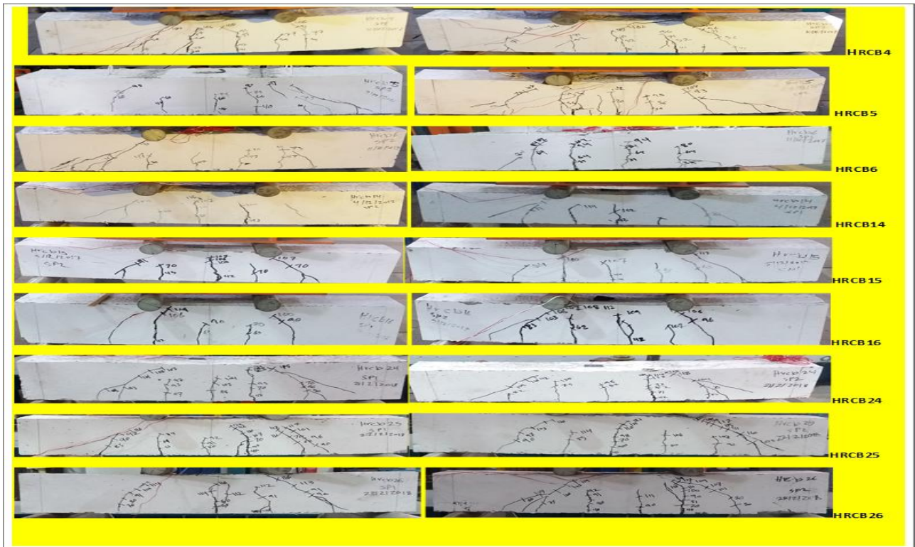
Fig 4 Crack patterns of tested beams at failure
