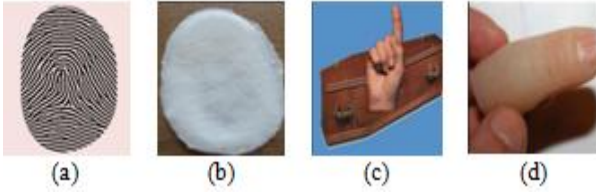
Fig. 2 Example of fake fingerprints. (a) reverse-engineered fingerprint image; (b) 2-D fake fingerprint using Silicone; (c) cadaver fingerprint; (d) synthesized 3-D fake fingerprint [3]
