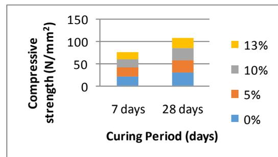
Fig. 4 Comparison chart for compressive strength of concrete cubes
