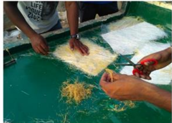
Fig. 4 Sample grinding for wet hand layup process
