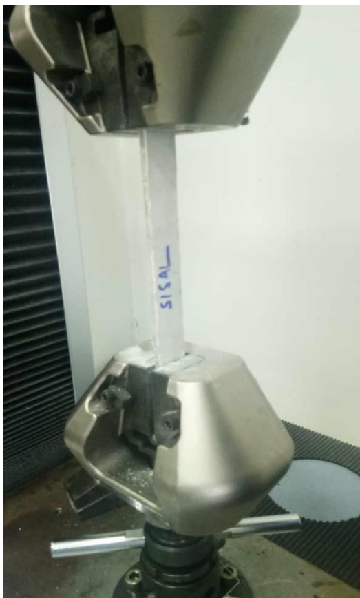
Fig. 5 tensile test on sisal panel
