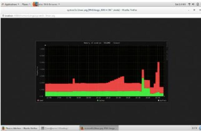
As we can see in the above graph a point is reached where the RAM usage was suddenly reached to 5GB and system get hanged due to this the system will go down and downtime occurs, all the processes running will abruptly and unexpectedly be stopped.
