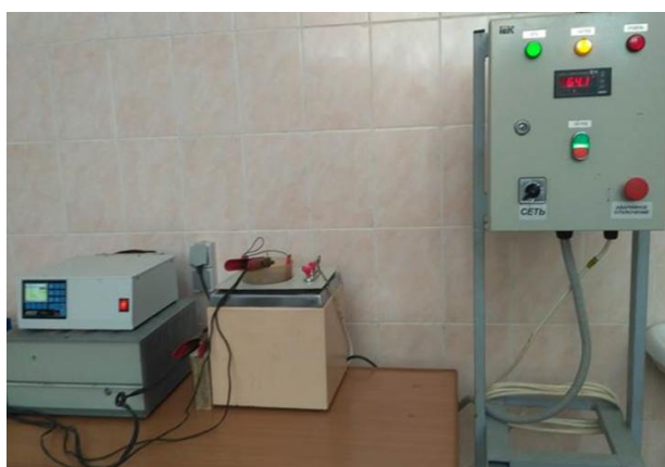
Fig. 1. Laboratory ultrasonic electroplating facility.
