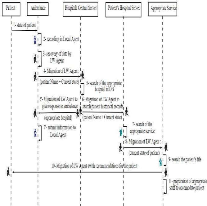
Figure 2. Diagram of data transmission for the first model
